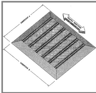
**SPLIT LOCATION:** If the unit exceeds the maximum width of 12', a split location must be noted on the template. Splits are joints where the mat or grid sections butt. We suggest locating splits away from heavy traffic areas.
